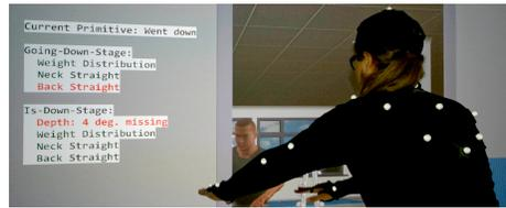
**Fig. 2.** The athlete is in the Is-Down-Stage. Here, he did not yet reach optimal depth (marked in red). During going down, PSP “Straight Back” was violated.
