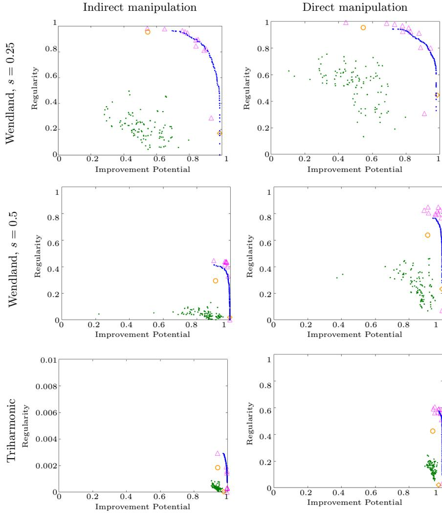
**Fig. 3.** The Pareto front (blue dots) and the initial random population (green dots) for the function approximation scenario. The magenta triangles are the results of the weighted single-objective optimization described in Section 6. Heuristic setups generated with Lloyd (orange circle) or OLS (orange diamond), discussed in Section 7, result in very regular setups or setups with a very good improvement potential.
