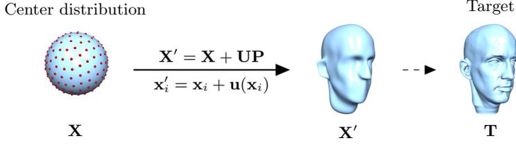
**Fig. 1.** The RBF deformation  $\mathbf{u}$  transforms the initial mesh  $\mathbf{X}$  to  $\mathbf{X}'$  by translating each vertex  $\mathbf{x}_i$  of  $\mathbf{X}$  by the displacement  $\mathbf{u}(\mathbf{x}_i)$ . The distribution of the RBF centers (red dots) is crucial for a high-performing fit of the mesh  $\mathbf{X}$  to the target  $\mathbf{T}$ .
