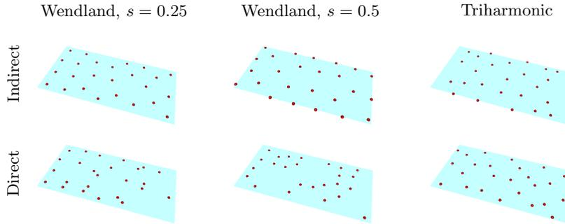
**Fig. 4.** Optimized center distributions towards regularity are uniform for indirect manipulation (top) but tends to be unintuitive for direct manipulation (bottom).
