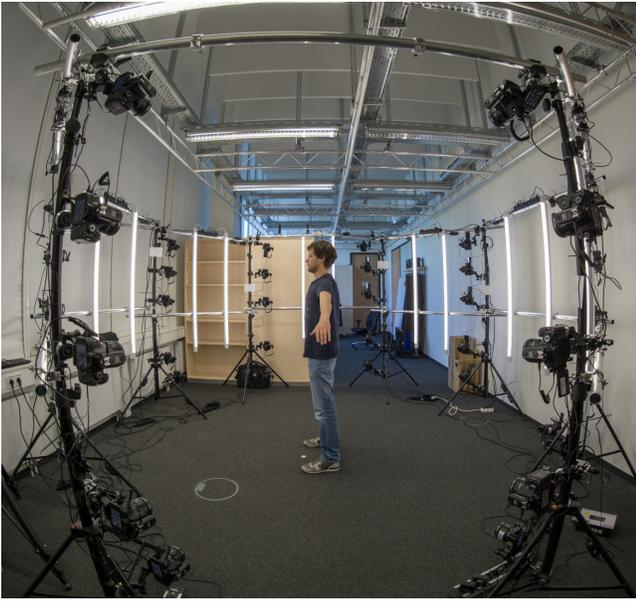
**Figure 9: The developed photogrammetry rig used to scan the full bodies.**
