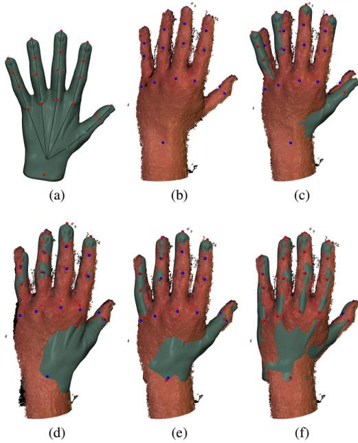
**Figure 8:** We fit a template model (a) to the point cloud (b) by using landmarks (red and blue dots). For initial alignment and adaption of the posture we perform rigid ICP (c) alternating with inverse kinematic (d). Afterwards we fit the shape of the template model based on landmarks (e) and closest point correspondences (f).
