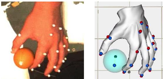
**Figure 20:** Comparison of the real human subject performing a grasping motion (left) and the animation of the virtual hand model reconstructed by our system (right). The animation is best appreciated in the accompanying video.
