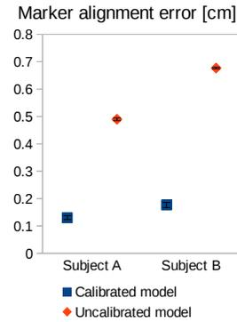
**Figure 17:** Average marker alignment error using calibrated and uncalibrated models for two subjects across all captured data. The error is significantly improved by our user-specific model calibration. The slightly larger error for Subject B is due to larger hands.
