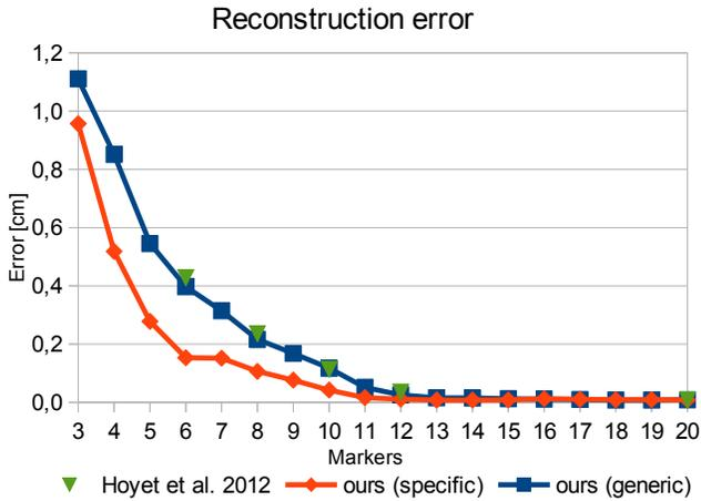
**Figure 11:** Average reconstruction error using marker sets of varying sizes for grasping motions. Using marker layouts specifically generated based on grasping input motions the reconstruction error is lower than when using a layout based on generic motions. The manually selected marker layouts of Hoyet et al. [Hoyet et al. 2012] produce similar results to our automatically generated generic layouts.
