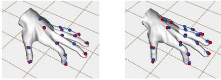
**Figure 19:** The alignment between the model’s virtual markers (blue) and the captured marker data (red) is more accurate with our user-calibrated model (left) than the uncalibrated template model (right). Small discrepancies with the calibrated model are due to differences between real hand deformations and our simple LBS deformation model.
