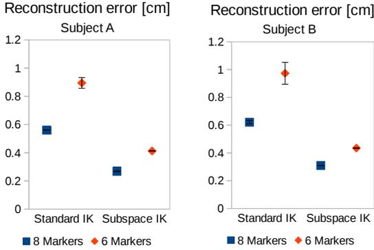
**Figure 15:** Comparison between the reconstruction error for reduced marker layouts using standard IK and subspace IK. Reduced marker sets perform within 5 millimeters accuracy using our subspace IK approach. The slightly larger errors for Subject B are due to larger hands.
