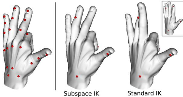
**Figure 3:** Full and reduced marker sets and reconstructed hand postures with standard inverse kinematics optimizing for all joint angles and subspace inverse kinematics optimizing for reduced subspace parameters. While the standard approach cannot articulate the markerless fingers, the subspace approach captures the correlations between fingers and articulates them using the reduced marker set.
