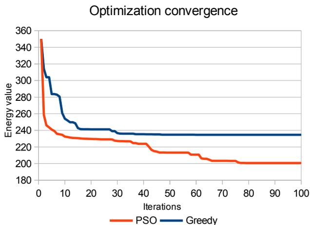
**Figure 9:** Example for the energy minimization convergence of our PSO method compared to a greedy approach with identical initialization. While the greedy approach converges to a suboptimal local minimum after about 50 iterations, our stochastic optimization minimizes the energy faster and achieves a better result.
