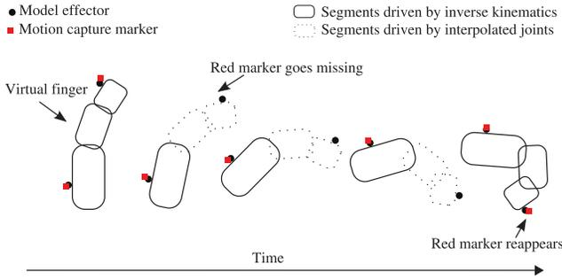
**Figure 4:** A virtual finger is shown as it moves through space and is bent. In the second rendering the motion capture marker is no longer visible. Once the marker reappears, inverse kinematics are computed in order to verify that the posture is possible and then the intervening frames in which the marker was missing can be updated using interpolation of the affected joints.
