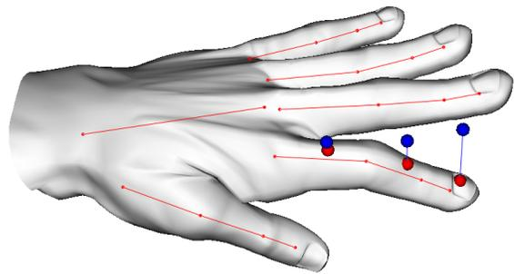
**Figure 2:** Hand model and its underlying skeleton. Also shown are three exemplary markers on the hand model (red) that are constrained to move towards their target positions (blue) using inverse kinematics.
