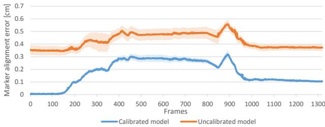
**Figure 18:** Marker alignment error using calibrated and uncalibrated models for one movement sequence by Subject B. The graph shows both the mean marker error and the variance across all markers for each frame. Our calibration improves upon both the mean and the variance of the marker alignment error.
