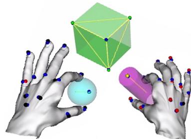
**Figure 13:** Synchronous tracking of two hands manipulating a number of rigid objects. Our system automatically clusters the raw marker point cloud and fits generic model templates to the data.
