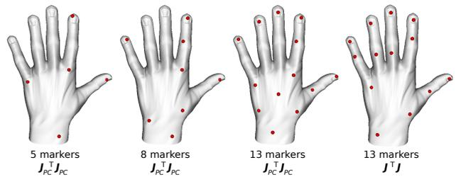
**Figure 5:** Marker layouts of different sizes for a precision grasp movement involving the index finger and thumb. The rightmost layout with 13 markers was computed using the full Jacobian  $\mathbf{J}$  for the condition number metric, whereas the others were computed using the reduced Jacobian  $\mathbf{J}_{PC}$ .
