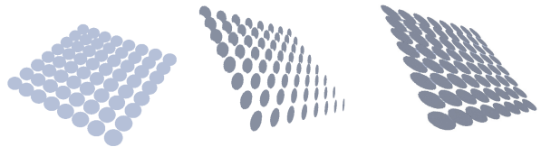
Figure 6. In order to show the effect of depth correction the z -buffer of the left scene has been re-projected using the techniques of [12]. While splats rendered without depth correction (center) have constant depth, like being parallel to the image plane, per-pixel depth correction solves this problem and avoids blending artifacts (right).
