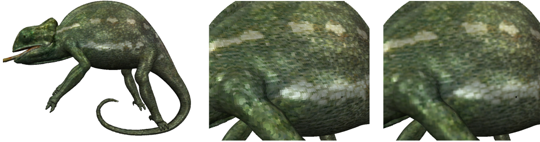
Figure 5. Splat filtering including per-pixel normalization results in high quality image reconstruction. This effect becomes especially visible in the case of high frequency textures. While in the left unfiltered image alias-problems appear, the splat filtering on the right provides a smooth result.
