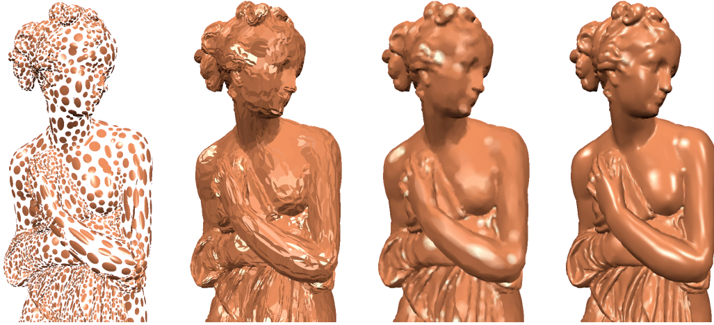
Fig. 12. Comparing different rendering techniques for a simplified model of a scanned statue: naïve splatting without filtering is comparable to flat shading ( center left ), Gaussian blending corresponds to Gouraud shading ( center right ), Phong splatting yields the same quality as Phong shading for triangle meshes ( right ).
