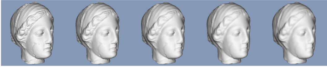
Figure 9: A series of successive smoothing operations on the Igea model. The model size is 134k points. A neighborhood of size 16 has been used for the MLS projections. Only MLS software code has been replaced by FPGA driver calls.
