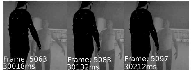
Figure 5: Example frames from one of the latency test videos (highest quality character with shadows). The left image shows the user’s arm approaching the lowest point. The image in the middle shows the turning point of the real arm, the picture on the right shows the turning point of the virtual arm, while the real arm already moves upwards.
