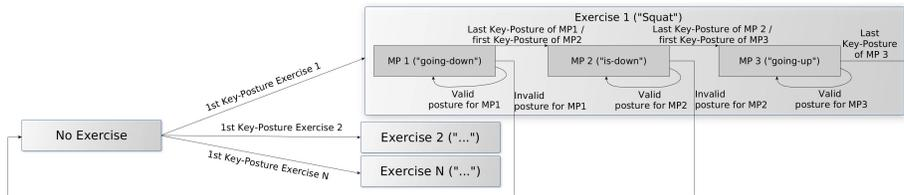
**Fig. 1.** State machine used to determine current action and Movement Primitive.
