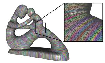
Fig. 19. Line Integral Convolution visualization obtained by anisotropically diffusing a random color signal along the maximum curvature direction.
