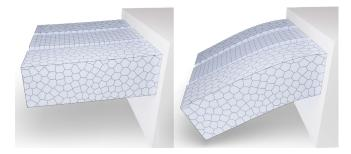
Fig. 20. Displacements due to gravity by linear elasticity with Young's modulus 5e+10 and Poisson ratio 0.4999 on differently tessellated bars consisting of tetrahedra, hexahedra, and Voronoi cells. The left figure shows the results for linear basis functions [Bunge et al. 2021] and the right for our quadratic basis.
