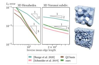
Fig. 14. *L*2 error in log-log scale of the Poisson system solved for Franke's test function on unit cubes with regular hexahedra (left) and subdivided Voronoi cells (center) in accordance to the Poly-Spline refinement (right).
