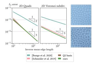
Fig. 13.  $L^2$  error in log-log scale of the Poisson system solved for Franke's test function on planar grids with quads (left) and subdivided Voronoi cells (center) in accordance to the needs of the Poly-Spline method (right).
