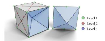
Fig. 6. Node positions for a refined cube. Parts of the mesh are detached for visualization purposes. All 2-faces are split into triangles using a virtual vertices. The volume is decomposed into tetrahedra by introducing a central virtual vertex which is connected to all face triangles. The nodes are colored according to their type.
