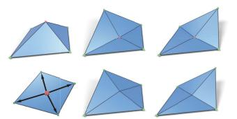
Fig. 3. Linear shape functions  $\psi_i$  on a refined quad element (top row) are combined to form a basis  $\varphi_i$  on the original polygon (bottom row).
