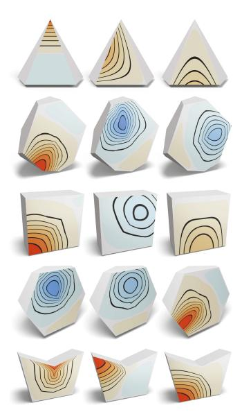
Fig. 8. Cross-sections showing our quadratic shape functions, for different polyhedra: While the shape functions are optimized for smoothness, they may exhibit small gradient discontinuities across virtual faces, visible as sharp corners along iso-curves. For tetrahedra (top), where we reproduce quadratic Lagrange shape functions, the functions are  $C^1$  inside the simplex.
