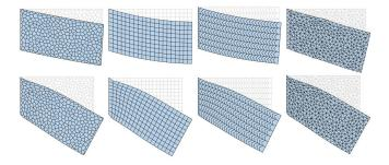
Fig. 17. Displacements due to gravity computed by linear elasticity with Young's modulus 1e+10 and Poisson ratio 0.4999 on differently tessellated 2D bars. The top row shows the results for linear elements [Bunge et al. 2020] and the bottom row for our quadratic basis functions.
