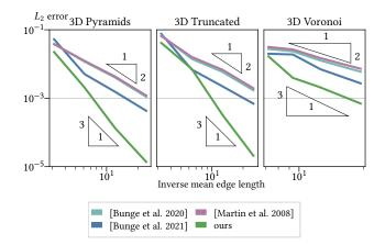
Fig. 12.  $L^2$  error in log-log scale of the Poisson system solved for Franke's test function on different tessellations of the unit cube. The tesselations are as follows: Pyramids (left), truncated cells (center), and Voronoi cells (right).
