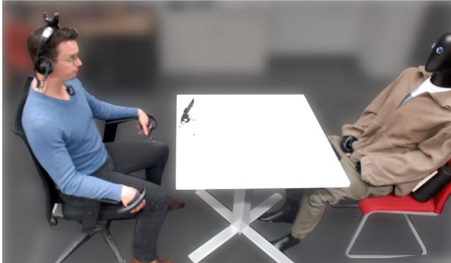
**Figure 2: Performance capture setup.** Actor facing a mannequin as target while equipped with head tracker, microphone, and hand controllers, with face tracker on table.
