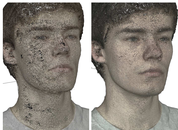
Fig. 2. Reconstructed point clouds from video frames (left) and images (right).
