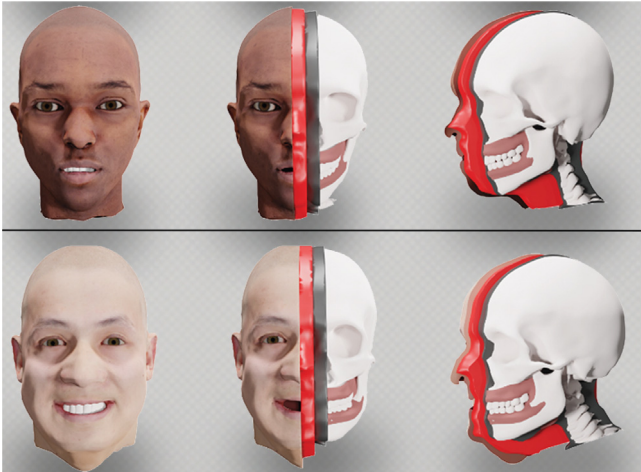
Fig. 6. Exemplary fits of the LHM components skull wrap, muscle wrap, and skull.
