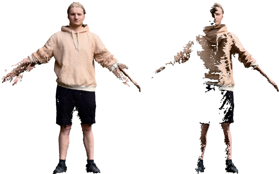
Figure 6.1: Point cloud from all images (left) and sub-scan capturing the left part of the subject (right). The full point cloud exhibits noticeable motion artifacts in both arms.
