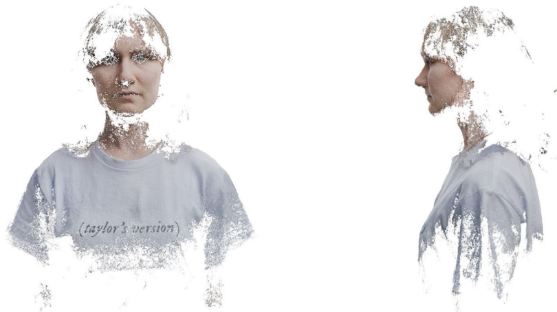
Figure B.25: The point cloud generated by Agisoft Metashape [Agi25] for a female subject with loose hair. Due to windy conditions during the scan, the photogrammetry was unable to match hair features across the image sequence, resulting in only partial reconstructions.
