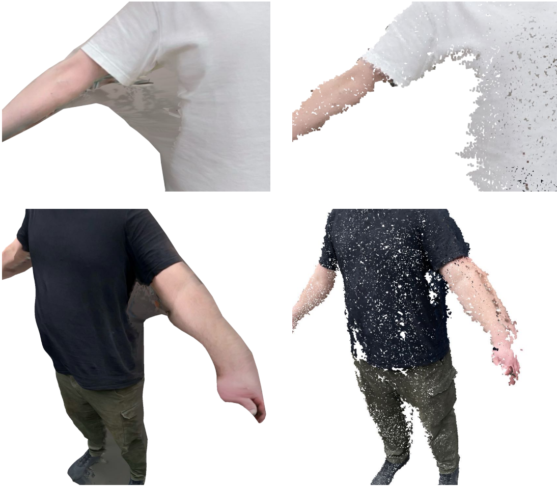
Figure 6.4: Comparison between the results of Apple’s photogrammetry API (left, [App23b]) and Agisoft Metashape (right, [Agi25]) on two exemplary sub-scans. Apple’s photogrammetry API produces a triangle mesh; Agisoft Metashape offers more options, among them the option to produce point clouds. The results show that Apple’s photogrammetry API attempts to fill in missing information from the sub-scan sequences to create a watertight mesh; however, this creates artifacts (e.g., area below the arm in the upper example, thickness of the arm in the lower example). In contrast, the results from Agisoft Metashape show that Metashape does not fill in the missing information. In our use case, the behavior of Metashape is the preferred one, as our intention is to reduce the amount of artifacts with our sub-scans, not increase them.
