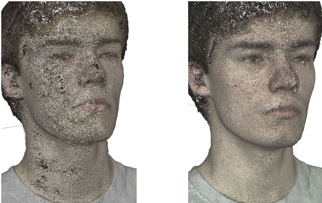
Figure 5.3: Point clouds reconstructed via photogrammetry from video frames suffer from compression artifacts (left). The higher quality of individually captured images yields more accurate point clouds (right).
