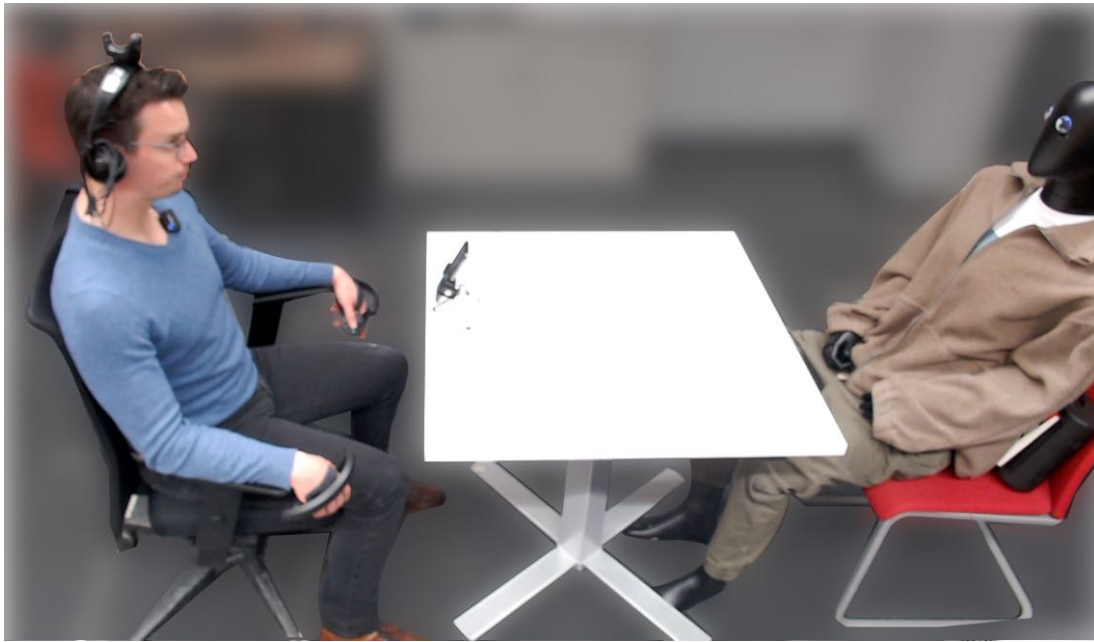
Figure 11.2: Performance capture setup. Actor facing a mannequin as target while equipped with head tracker, microphone, and hand controllers, with face tracker on table.
